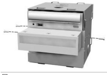
**Note:** If you removed the accessible device cage, replace it. Secure the device cage with the screw.
